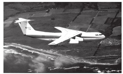
▼ FIGURE 15.5 The NASA Kuiper Airborne Observatory.
